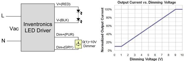
**Note:** If 0-10V dimming is not used, Dim + can be open.
